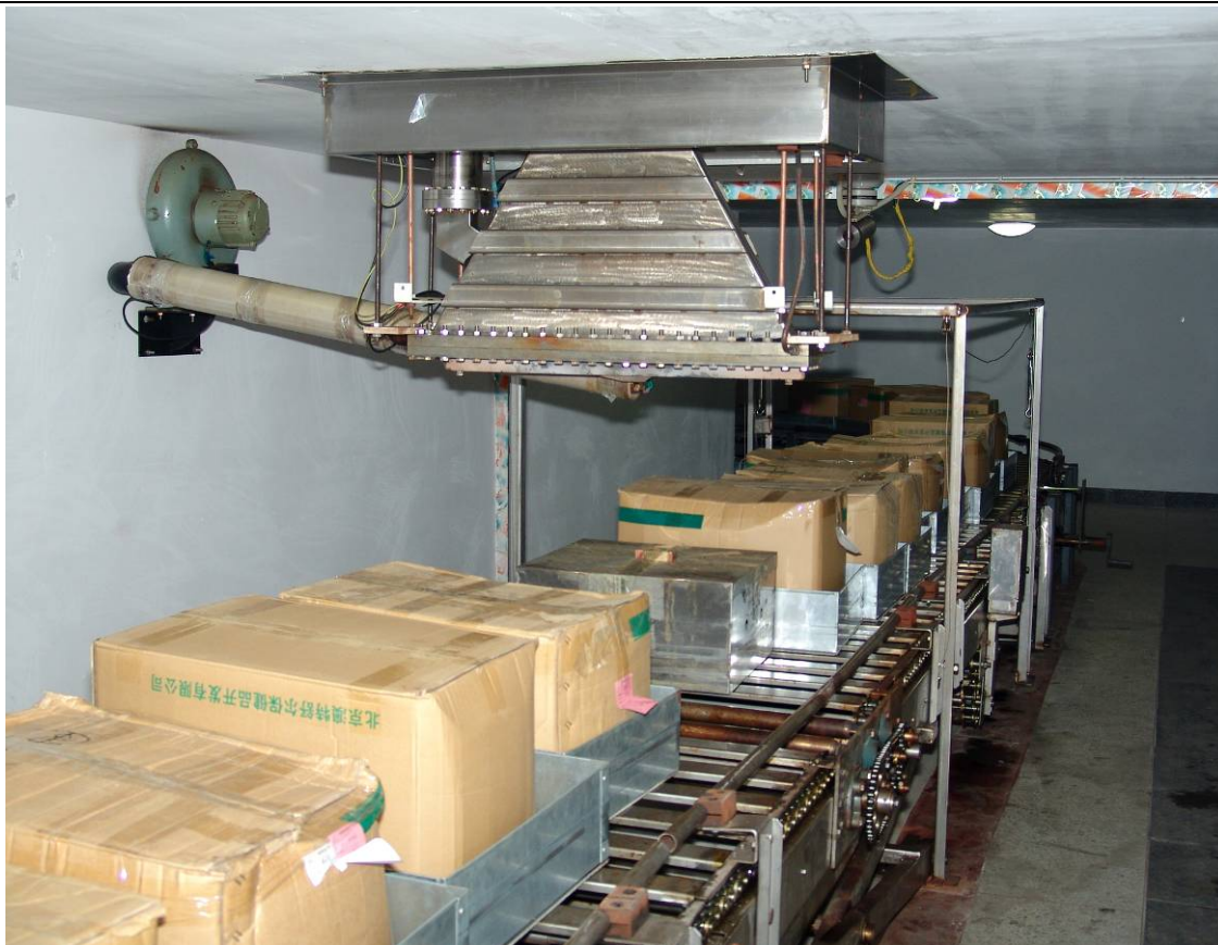
束下输送系统 delivery system under the Beam
