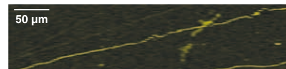
Large area (500 µm in X) StreamLine Plus image showing very long continuous carbon nanotube (CNT). Y resolution is 500 nm, X resolution is 5 µm.
